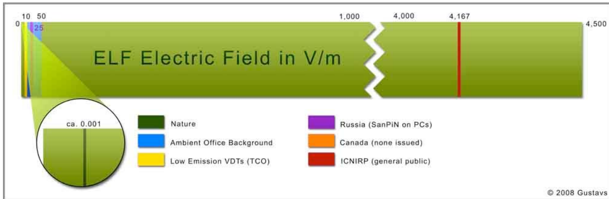
Figure 2: ELF Electric Field Levels and Exposure Limits
